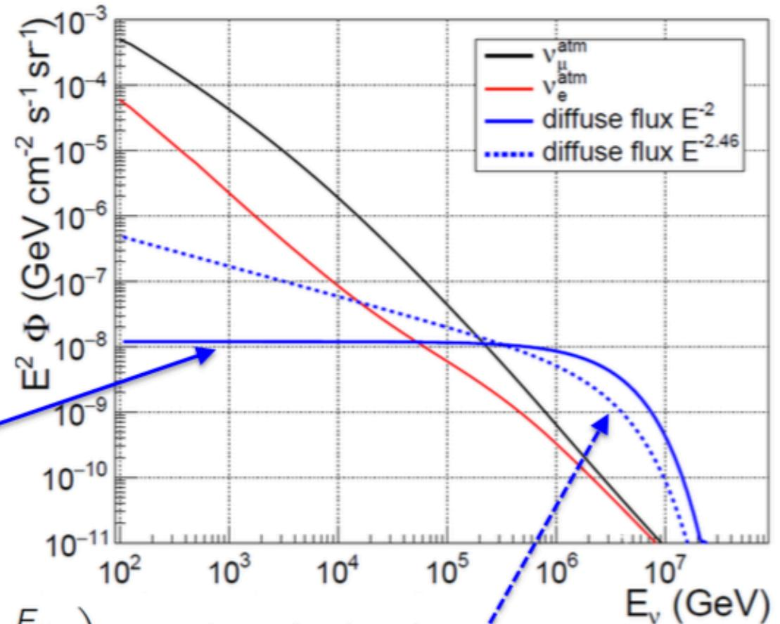
$$\Phi(E_\nu) = 1.2 \times 10^{-8} \cdot \left(\frac{E_\nu}{\text{GeV}}\right)^{-2} \cdot \exp\left(-\frac{E_\nu}{3 \text{ PeV}}\right) \text{ GeV}^{-1} \text{ cm}^{-2} \text{ s}^{-1} \text{ sr}^{-1}$$
